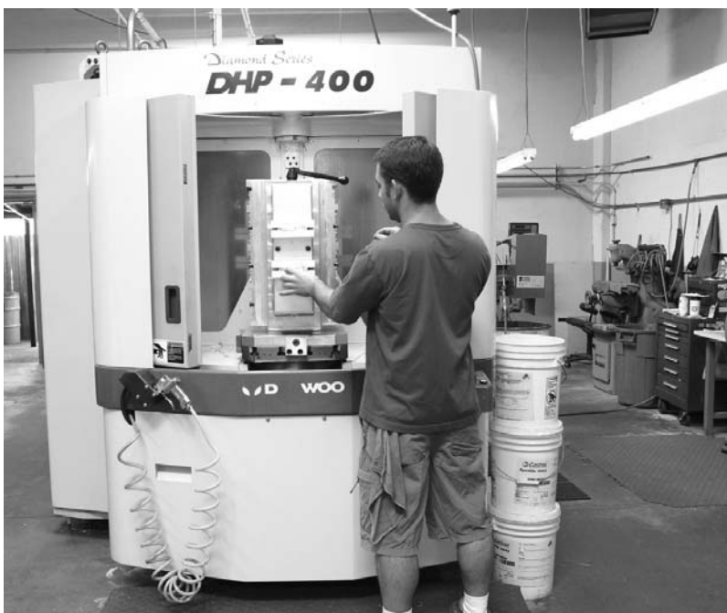
Mike Harrison, CNC operator, loads parts into one of two Daewoo DHP-400, dual-pallet horizontal machining centers operated by Wolf's Precision.
