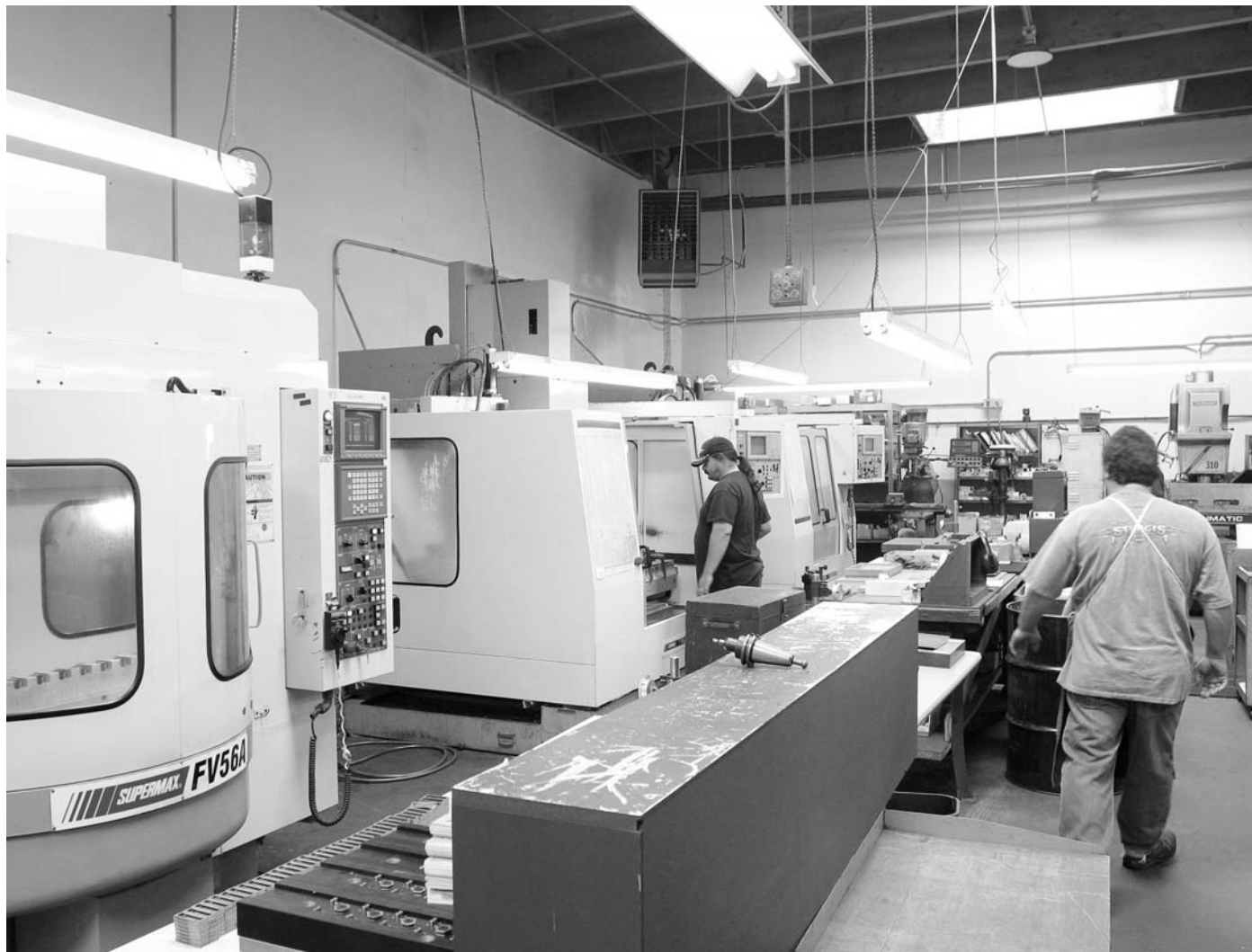
Line up of YCI machining centers used by Wolf's Precision Works, Inc. to machine copper tungsten carriers. The service is so tough the machines have to taken down once a year to clean out the copper tungsten powder that accumulates and causes the pallets to get out of level.
